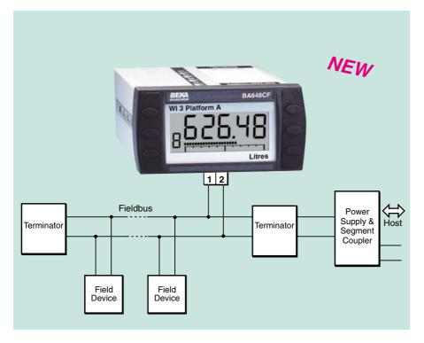
The BA648CF-P PROFIBUS Indicator is a general purpose instrument that can display up to eight fieldbus process variables. A numeric annunciator on the left hand side of the screen shows which variable is being displayed. This version of the indicator supports PROFIBUS PA protocol; for FOUNDATION<sup>™</sup> fieldbus systems an alternative version is available – please see BA648CF-F FOUNDATION<sup>™</sup> fieldbus datasheet.
